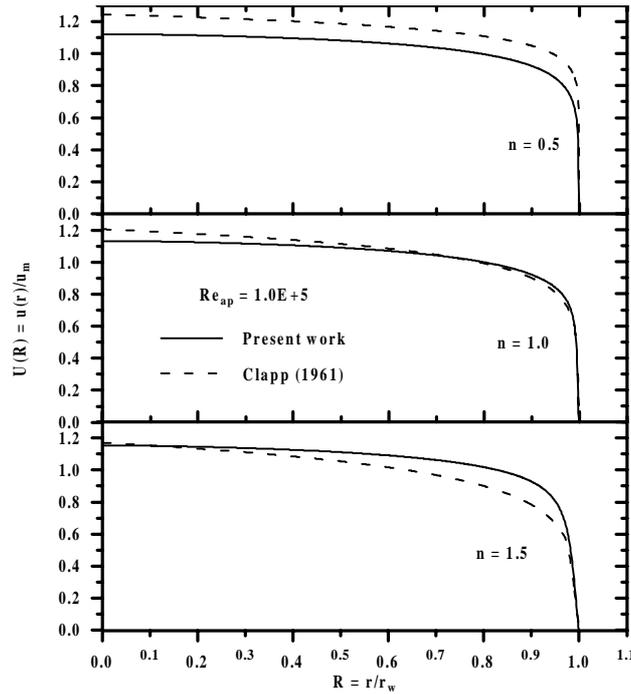
Figure 3. Effect of the parameter  $n$  on the turbulent velocity profiles for  $Re_{ap} = 10^5$ .
