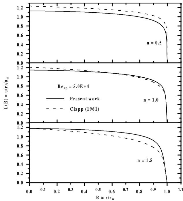
Figure 2. Effect of the parameter  $n$  on the turbulent velocity profiles for  $Re_{ap} = 5 \times 10^4$ .
