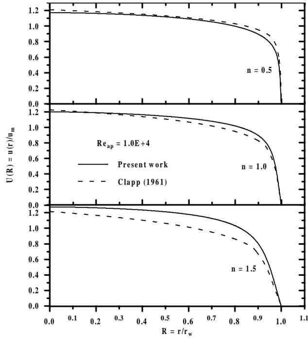
Figure 1. Effect of the parameter  $n$  on the turbulent velocity profiles for  $Re_{ap} = 10^4$ .
